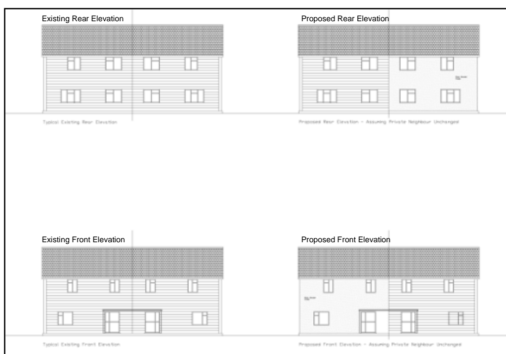
Figure 4 - Typical proposed and existing front and rear elevations. Please note that this elevation is typical of No.8 which is attached to a privately owned dwelling whose elevation will remain cladded. The other dwellings with new render will match the attached dwelling.
